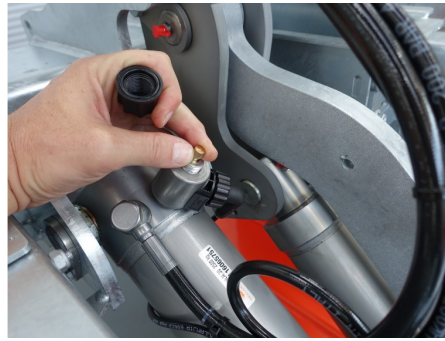
Self-lock valves with manual override
